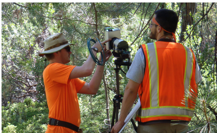
UMass Boston doctoral students set up a canopy biomass lidar in Sierra National Forest, California.
